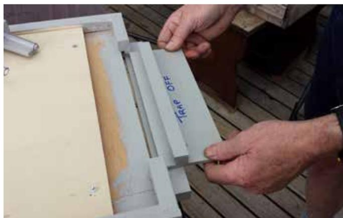
Inserting the entrance for putting the pollen trap in the TRAP OFF position.
